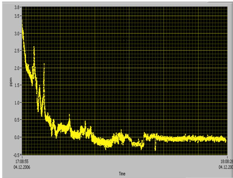
Calibration curve for H<sub>2</sub>CO concentration measurements
