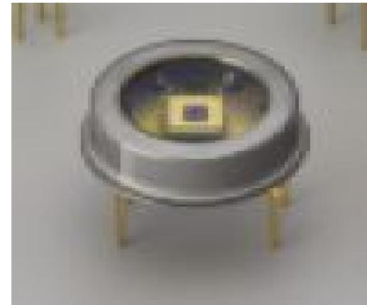
**View of laser module with collimator**
