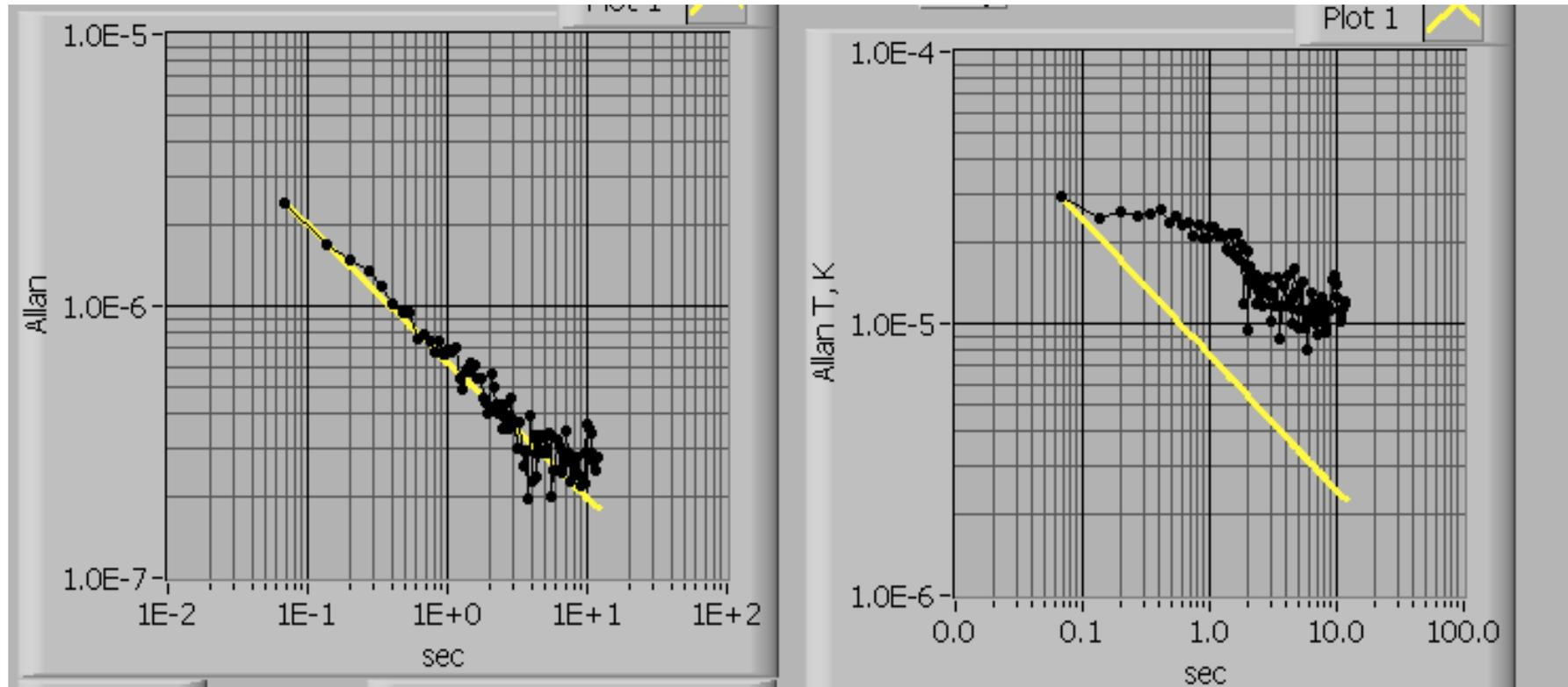
Minimum detectable absorption (left) and temperature stability (right)
